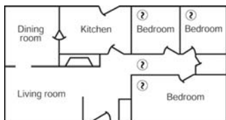
Figure 2: A SMOKE ALARM SHOULD BE LOCATED BETWEEN THE SLEEPING AREA AND THE REST OF THE DWELLING UNIT AS WELL AS IN EACH BEDROOM.
